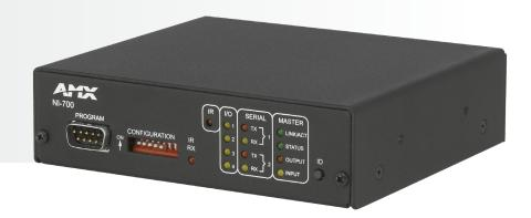
The NI-700 unit is geared to meet the specific control and automation needs of a single room environment, in which both price and functionality are the driving requirements. The NI-700 is configured to control a limited number of video players, projectors, lights, thermostats, and other electronic equipment.
