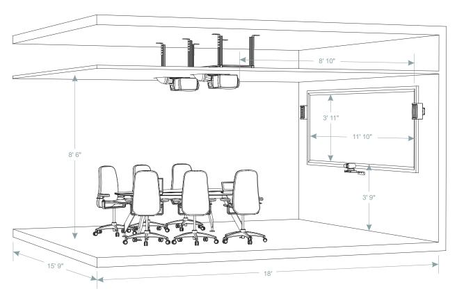
Dimensions indicate a typical installation and may be changed to match customer requirements.
