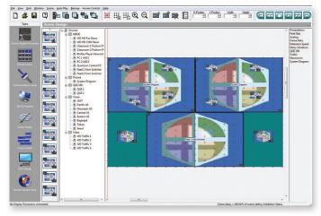
The virtual canvas provides a visual on-screen layout of the videowall, where windows can easily be added, sized, and positioned.
