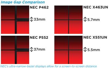
between two neighboring displays as thin as 5.5mm, close to 450% improvement compared to its previously revolutionary P Series displays.
