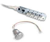
The X-Touch button interface is a 4-channel pushbutton interface with LED control and can be used in combination with industry-standard push buttons. It allows the connection of up to four buttons onto a single interface. This results in the connection possibility of up to 9 push buttons even on the smallest Xperience controller. Programmable LED output options are on, off, slow and fast blink.
