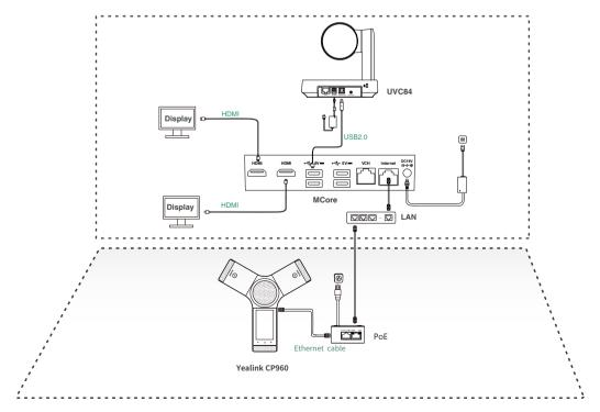
The IP phone should be powered by PoE adapter (54V/0.56A) or PoE switch. All devices are powered separately. The cable should be replaced at once if its skin is broken.
